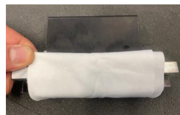
Fold the wipe around the printhead
